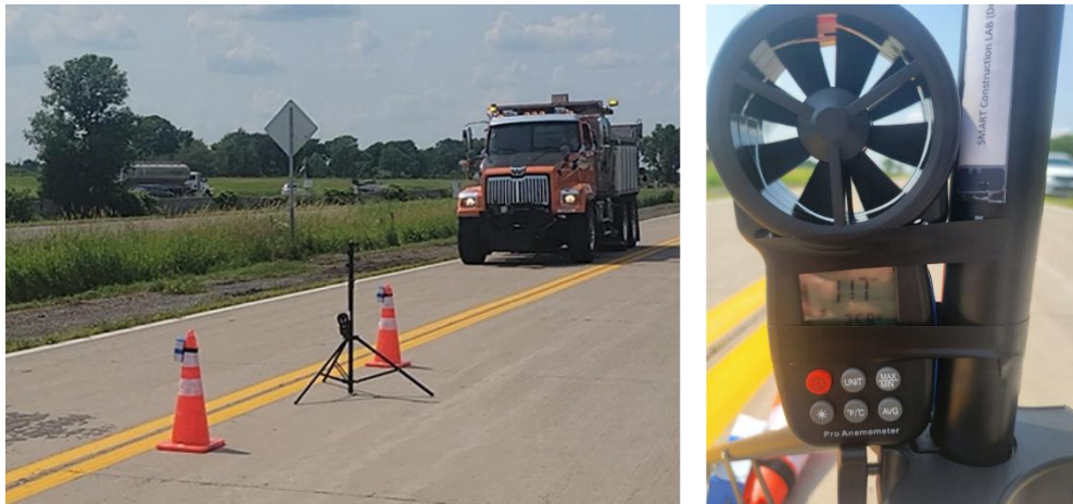
Figure 9. Wind-induced movement experiment. Left) Vehicle passing by traffic cones to generate wind disturbance; Right) An anemometer measuring wind speed to quantify its impact on cone displacement
